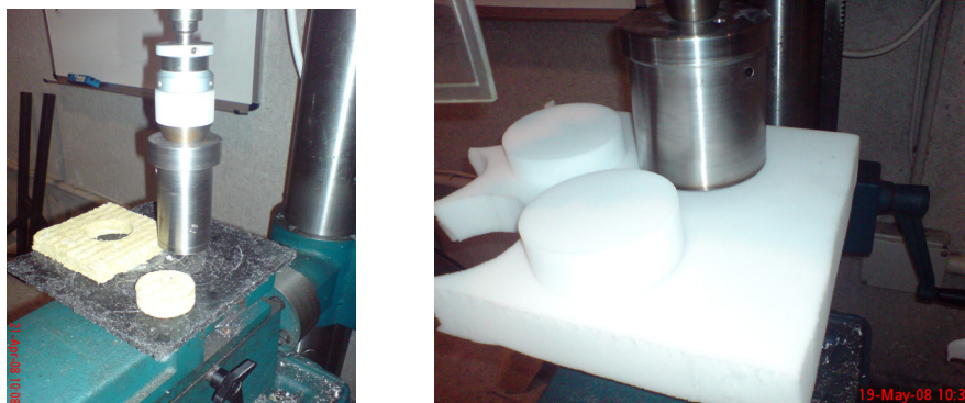
Figure 3: Rotating blade set up for cutting samples
