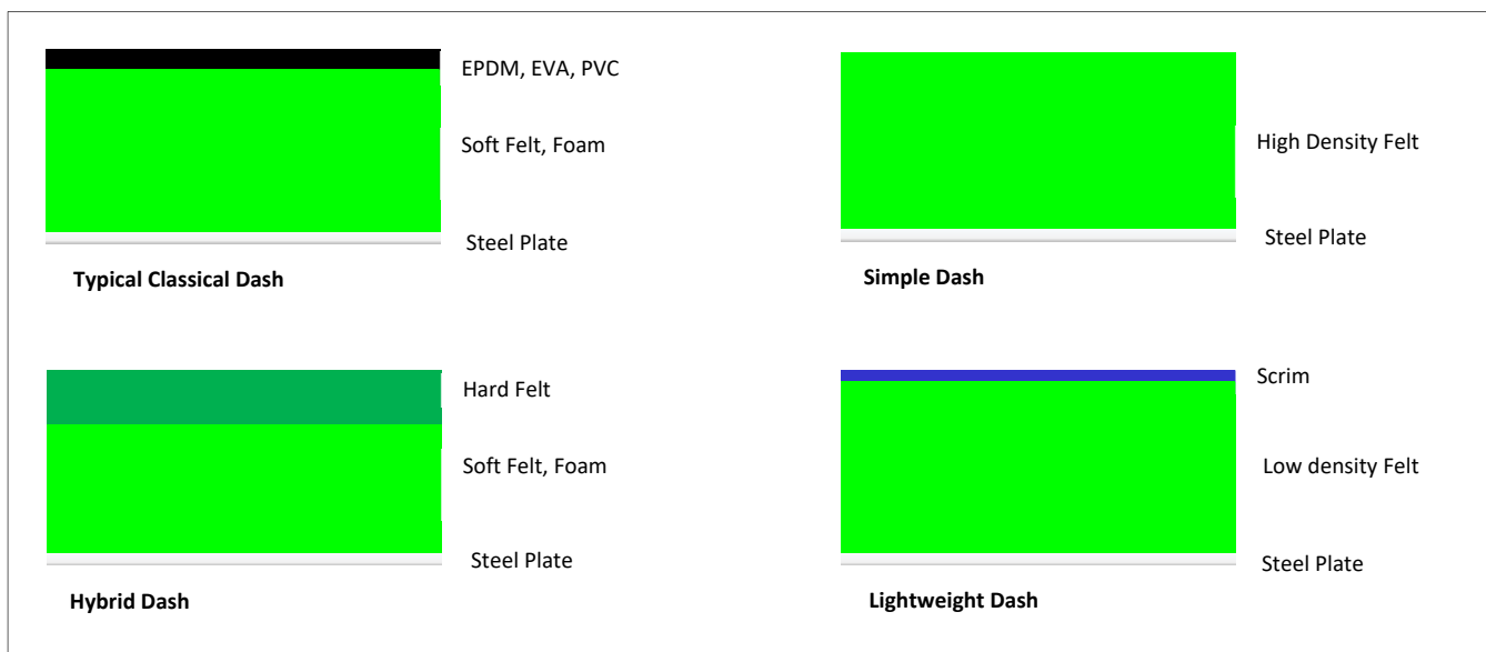
Figure 3. Layer wise configuration for different dash insulators
