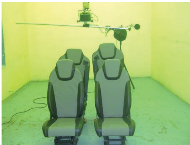
Figure 1. Test Set Up for Measurement of Reverberation Time and Sound Absorption of Automotive Seats in Reverberation Chamber.
