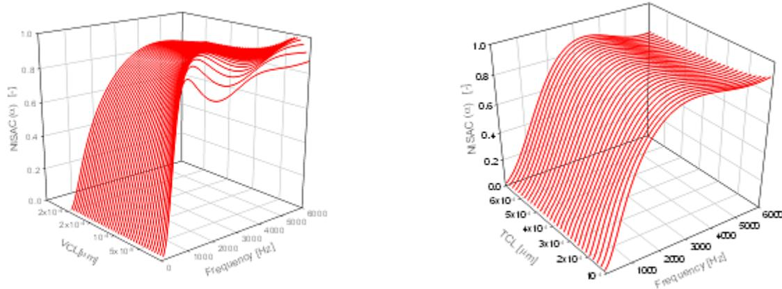
Fig. 4. Effect of characteristic lengths on Sound Absorption
