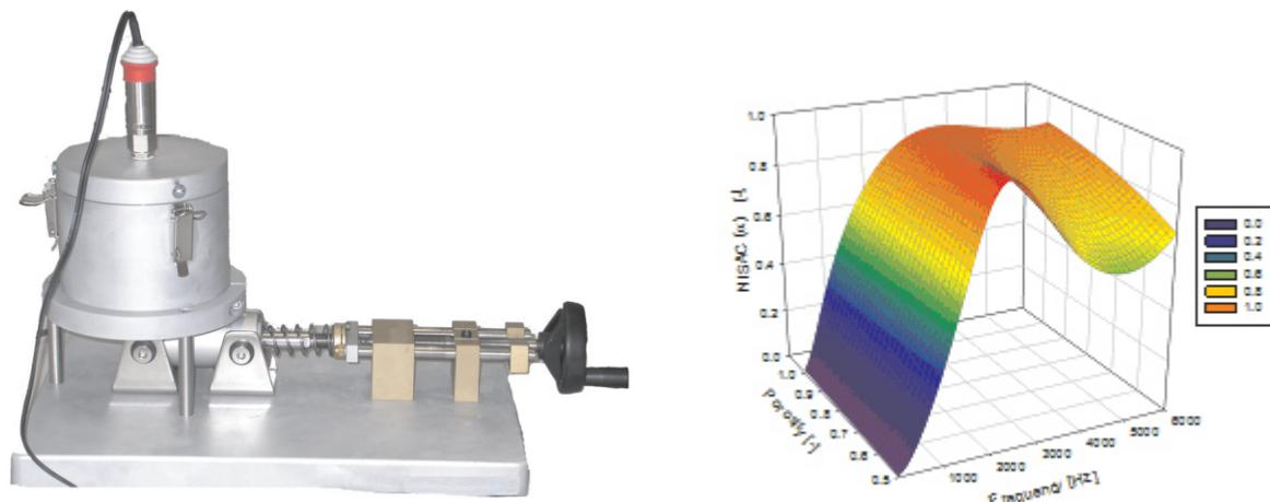
Fig. 1. Test rig for porosity measurement (ENDIF, Italy) and Effect of porosity on Sound Absorption
