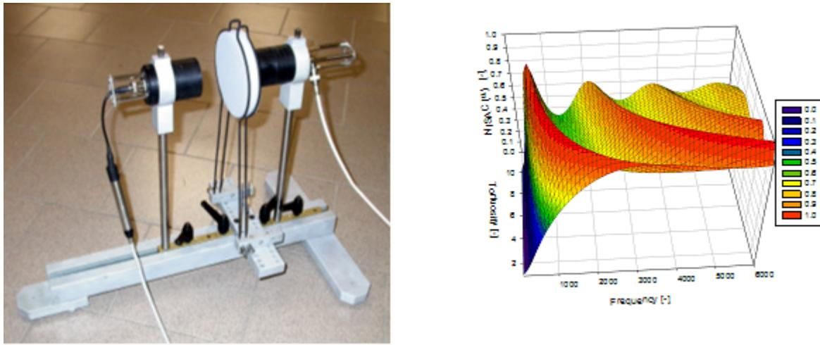
Fig. 3. Test rig for Tortuosity measurement (ENDIF, Italy) and Effect of tortuosity on Sound Absorption
