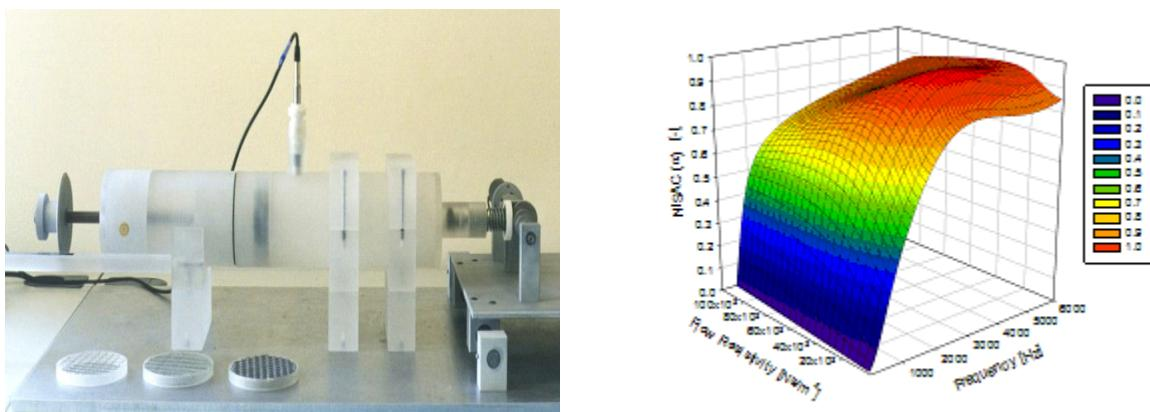
Fig. 2. Test rig for Flow resistivity measurement (ENDIF, Italy) and Effect of flow resistivity on Sound Absorption
