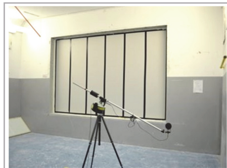
Partition Wall Testing in a Reverberation Suite
