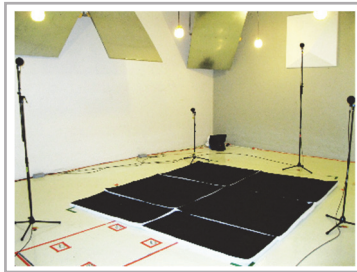
Sound Absorption Testing in a Reverberation chamber
