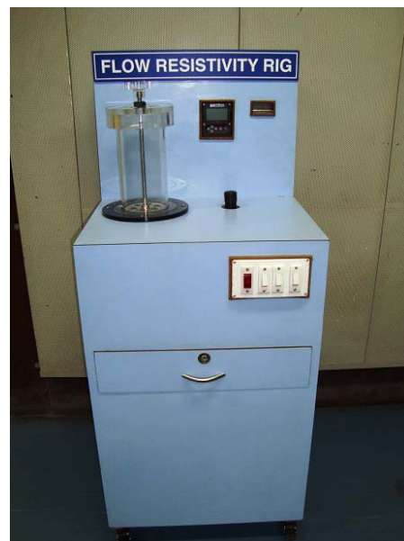
Fig. 2. Flow resistivity test rig
