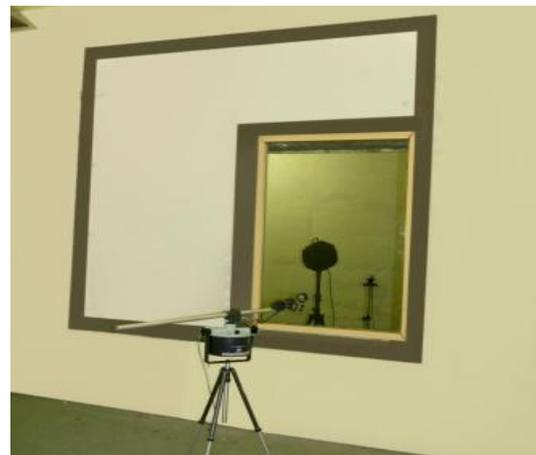
**Figure 6.** Reverberation Suite for Transmission loss Measurement
