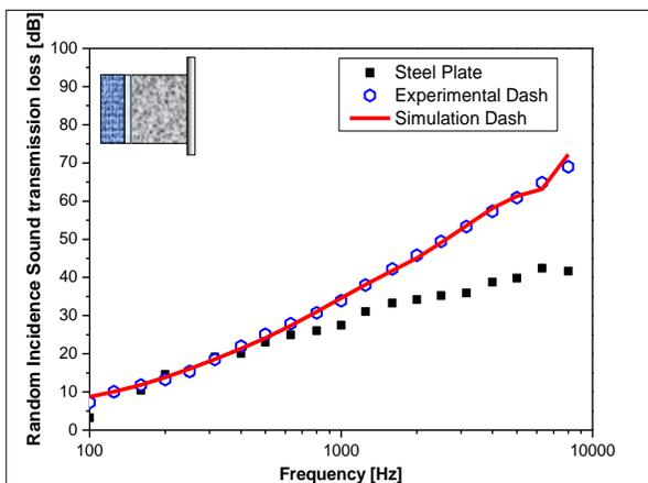
**Figure 13.** Comparison of experimental and simulated sound transmission loss for a typical dash Insulator
