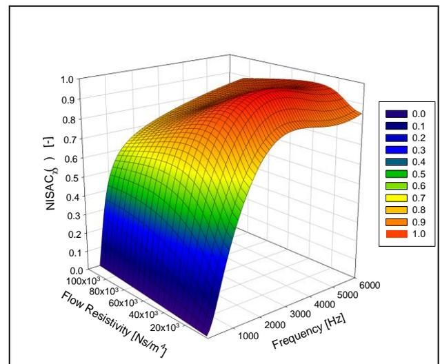
Figure 9. Effect of flow resistivity on sound absorption
