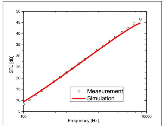
Figure 11. Comparison of Sound Transmission loss with simulation for 0.8 mm Steel Plate at Random Incidence
