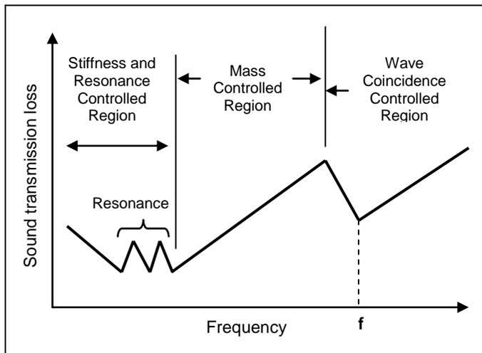
**Figure 2.** Sound Transmission Loss of single wall
