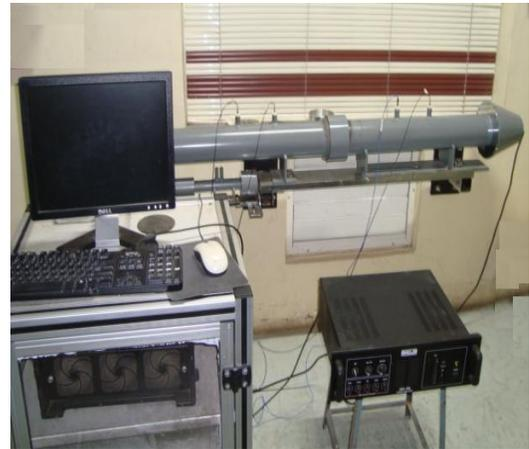
**Figure 5.** Four microphone Tube
