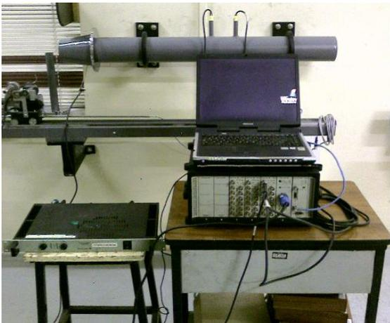
**Figure 3.** Two Microphone Impedance Tube
