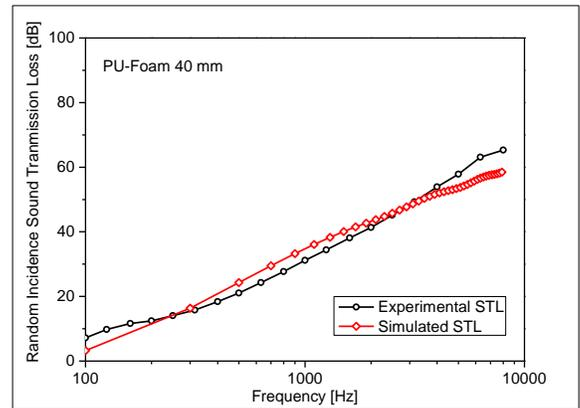
Figure 12. Comparison experimental and simulated Sound Transmission loss of PU Foam with Steel Plate at Random Incidence
