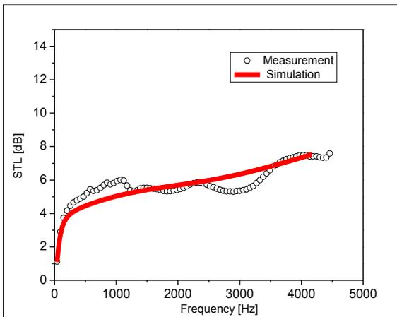
Figure 10. Comparison of Sound Transmission loss with predicted sound absorption for PU Foam at Normal Incidence
