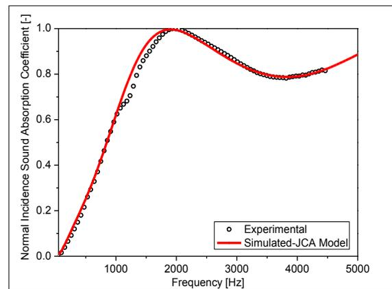
Figure 8. Comparison of Sound Absorption coefficients with predicted sound absorption for Polyurethane Foam at Normal Incidence
