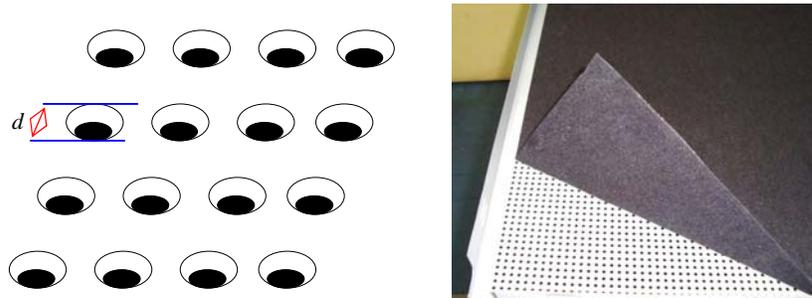
Figure 1: Geometry and Schematic of Metal Perforated Panel with Resistive Scrim
