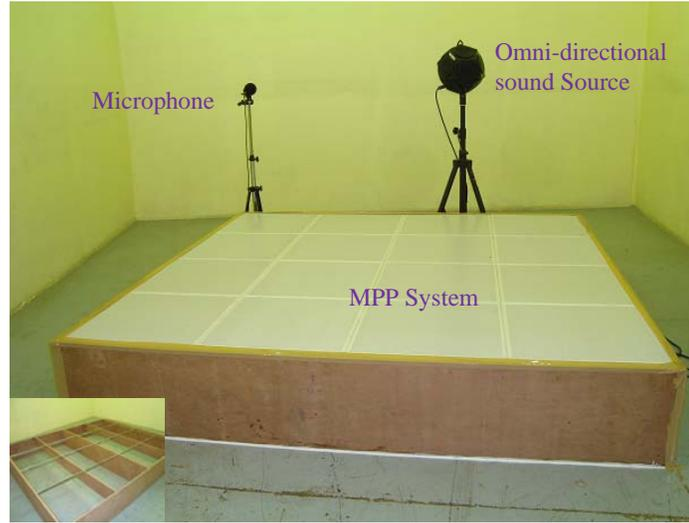
Figure X: Experimental Test setup for measurement of sound absorption coefficient in a Reverberation Room
