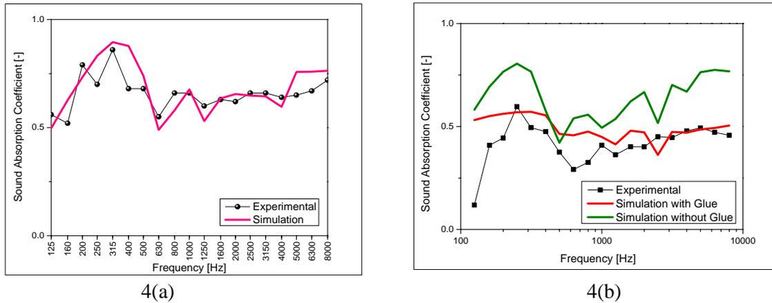
Figure 4: Comparison of predicted sound absorption coefficient with experimental sound absorption coefficient in a Reverberation Room
