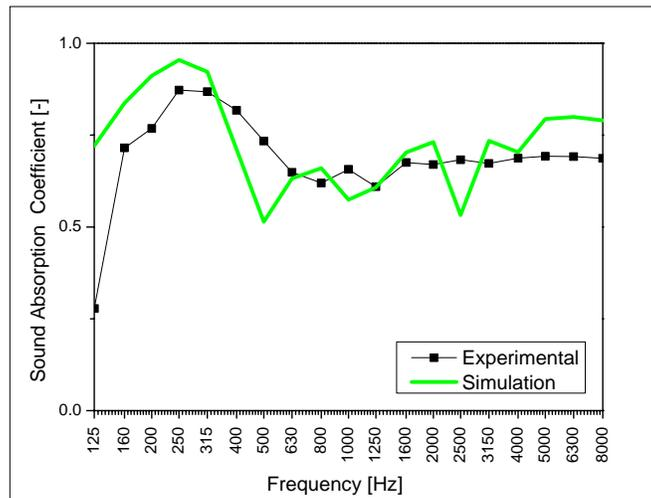
Figure 5: Comparison of predicted sound absorption coefficient with experimental sound absorption coefficient in a Reverberation Room
