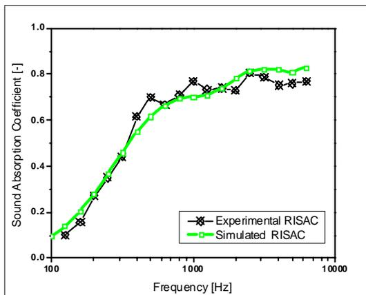
Fig. 5. Comparison of random in incidence sound absorption coefficient with simulation for cellular rubber
