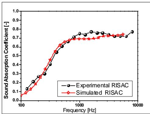
Fig. 3. Comparison of random in incidence sound absorption coefficient with simulation for PET felt
