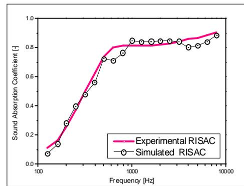
Fig. 4. Comparison of random in incidence sound absorption coefficient with simulation for polyester felt
