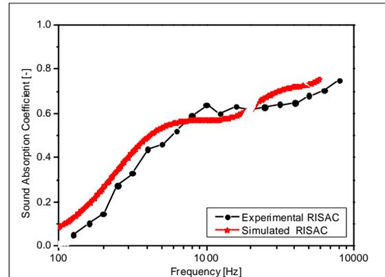
Fig. 6. Comparison of random in incidence sound absorption coefficient with simulation for PU foam
