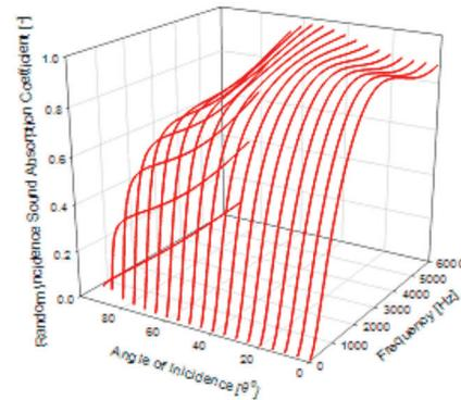
Fig. 2. Effect of Angle of incidence on sound absorption of PU foam
