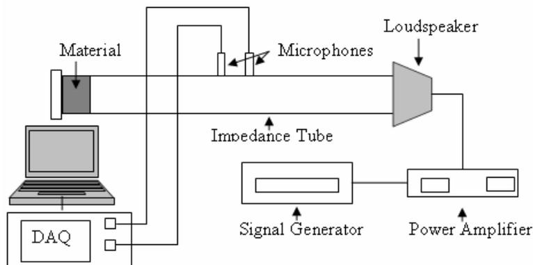
Fig. 3 Schematic of Experimental Setup for Normal Incidence Sound absorption coefficient
