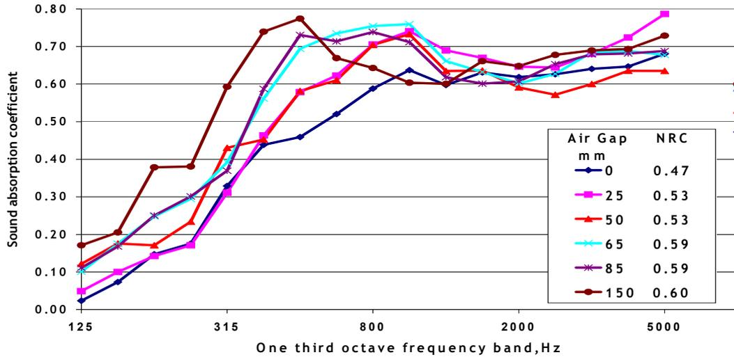
Fig 1: Effect of Air gap on random incidence sound absorption coefficient for Foam, 25mm thick and density 70 kg/m<sup>3</sup>
