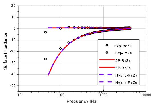
Fig: 5 Comparison of Surface Impedance for Glass Wool
