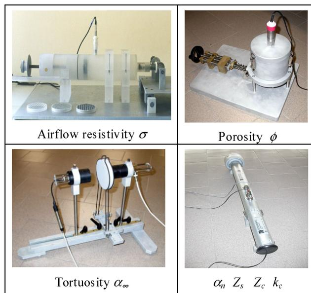
Figure 1 Experimental Test Rigs
