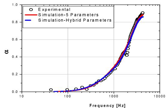
Fig: 2 Comparison of Sound Absorption Coefficient for Melamine foam
