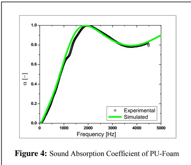
**Figure 4:** Sound Absorption Coefficient of PU-Foam
