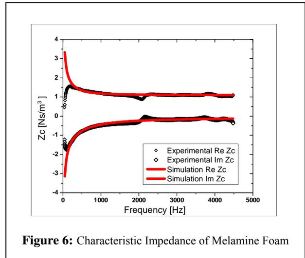
**Figure 6:** Characteristic Impedance of Melamine Foam
