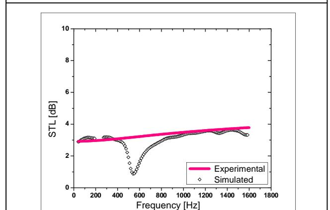
Figure 3: Sound Transmission Loss of Melamine Foam
