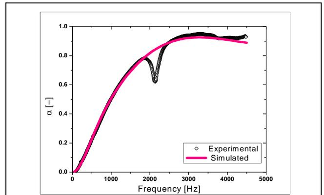
Figure 2: Sound Absorption Coefficient of Melamine Foam
