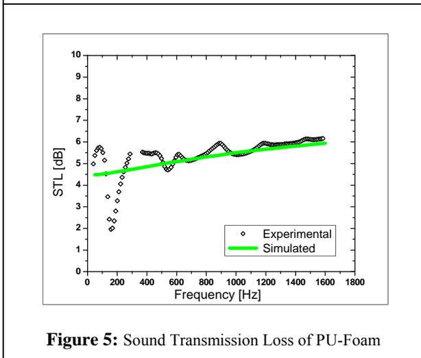
**Figure 5:** Sound Transmission Loss of PU-Foam
