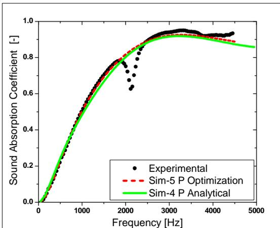
Fig. 4(a) - Comparison of measured and predicted Sound absorption coefficient for Melamine Foam.
