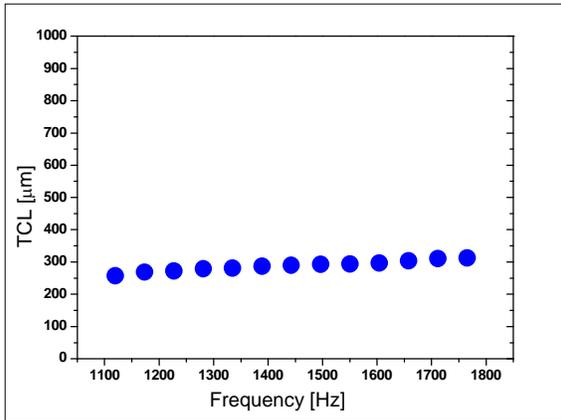
Fig. 3(a) - Computed Thermal characteristic length ( $\Lambda'$ ) for PU-foam.
