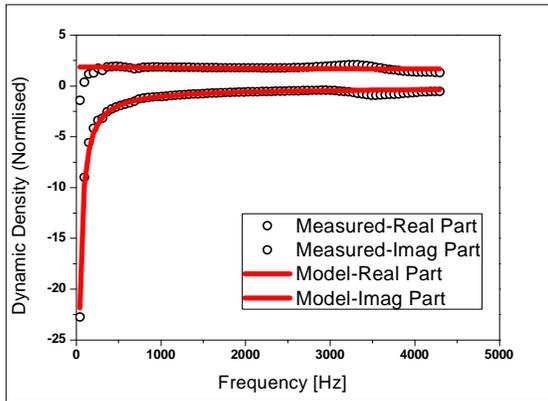
Fig. 5(a) - Comparison of measured and predicted dynamic density of for PU-foam
