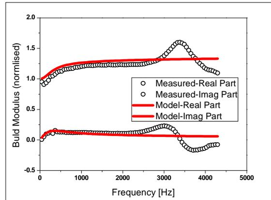
Fig. 5(b) - Comparison of measured and predicted bulk modulus of PU-foam
