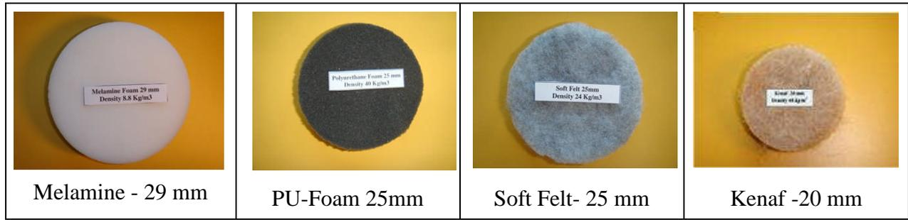
Fig. 1 - Samples of Materials used for Measurement of physical parameters.
