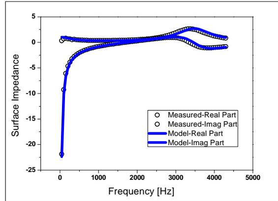
Fig. 3(b) - Comparison of measured and predicted Surface impedance for PU-Foam.
