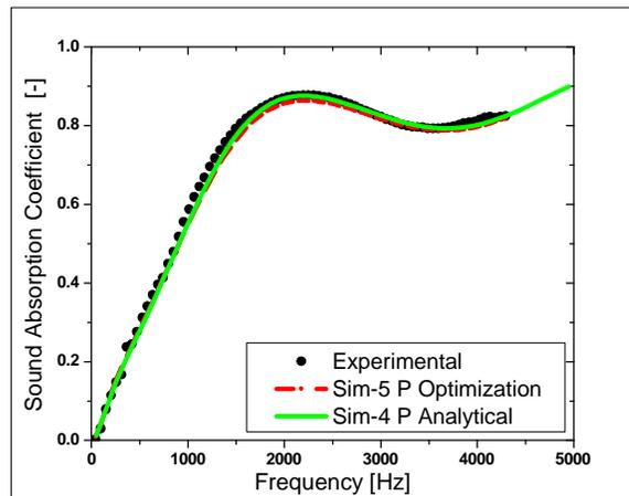
Fig. 4(b) - Comparison of measured and predicted Sound absorption coefficient for Polyurethane Foam.
