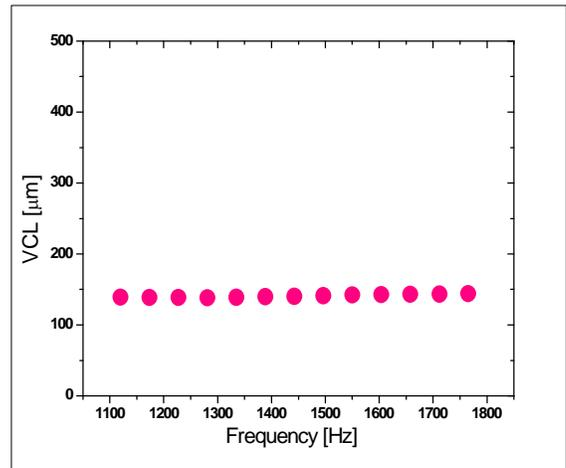
Fig. 2(b) - Estimated Viscous characteristic length ( $\Lambda$ ) for PU-foam.
