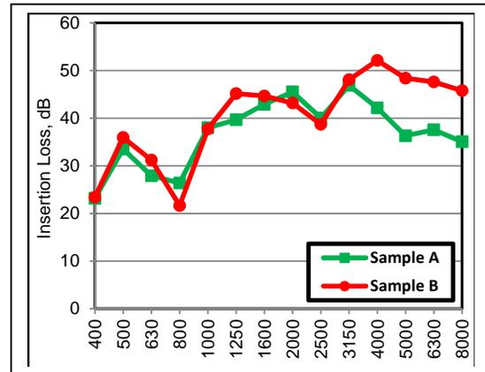
Figure 4: Comparison of Insertion Loss for expandable sealants
