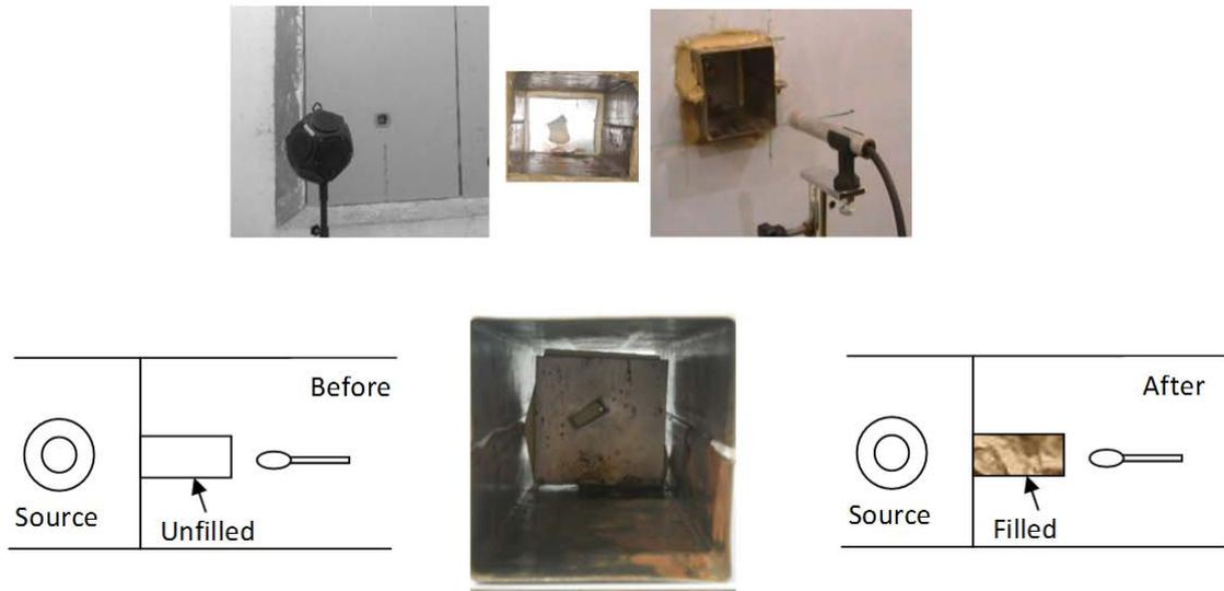
Figure 1: Test set for Insertion Loss of Cavity Filler Measurement
