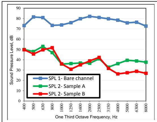
Figure 3: Sound Pressure Levels for Bare and Filled Channel
